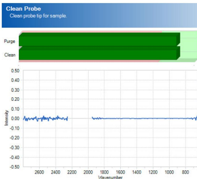
**Figure 6-28** 'Clean' sensor—Green indicator bars and flat spectral line
