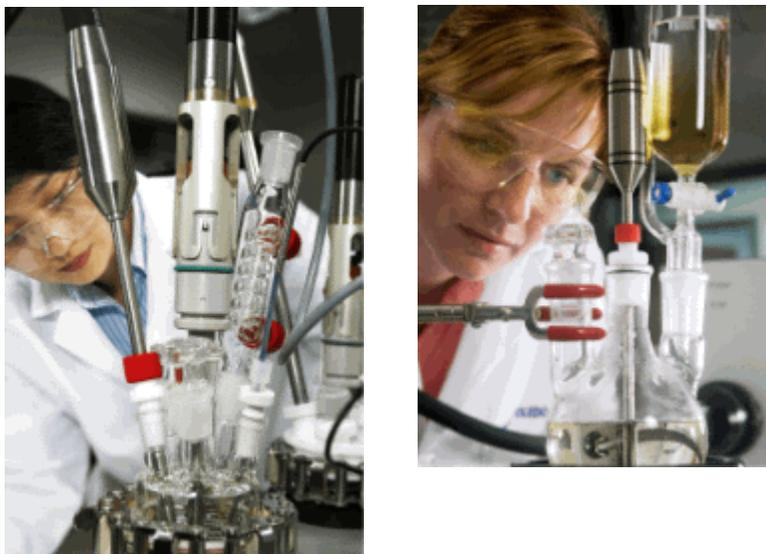
**Figure 6-23 DS FiberConduit with adapter in common reaction vessels**
