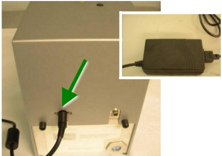
Figure 5-2 ReactIR 15 power cord connection on back panel (inset shows transformer)
