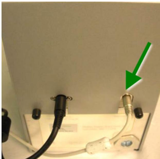
**Figure 5-3 ReactIR 15—Communications cable connection on back panel**
