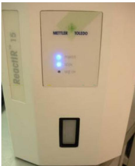
Figure 5-8 Power and Scan LEDs
