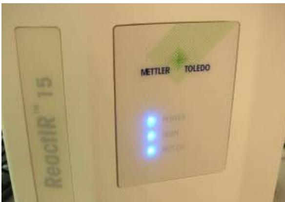
Figure 5-9 Power, Scan, and MCT OK LEDs
