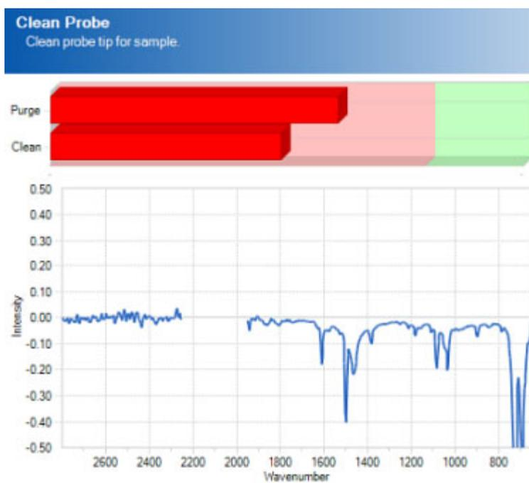
Figure 6-27 'Dirty' sensor—Poor cleaning method and subsequent collection of new background
