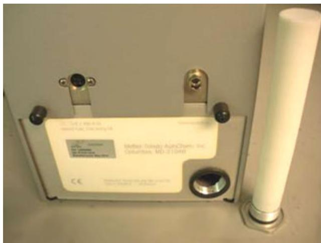
**Figure 7-35 Desiccant cartridge removed**
