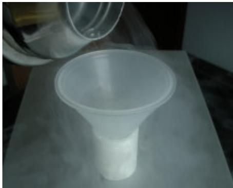
**Figure 6-13** Filling Dewar with liquid nitrogen to cool the detector
