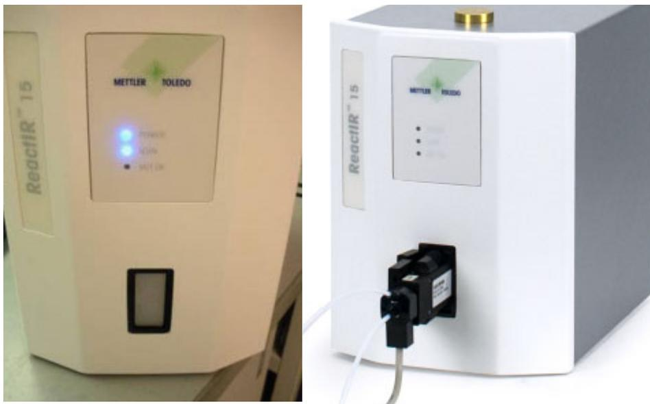
**Figure 5-5 Connecting DS Micro Flow Cell sampling technology**
