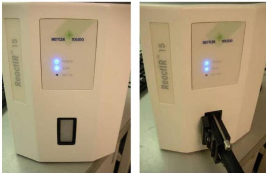
**Figure 5-4 Connecting DS FiberConduit sampling technology**
