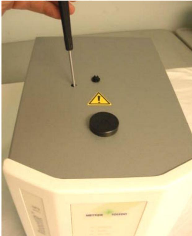
**Figure 6-14 Preamp adjustment on ReactIR 15**
