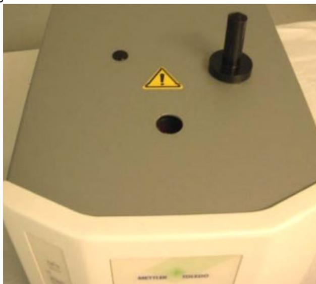
Figure 6-12 Liquid nitrogen fill port on ReactIR 15—Plug removed
